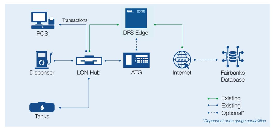
The DFS Edge service uses encrypted http(s) to send wetstock data to Dover Fueling Solutions. This can also be via a VPN if preferred.
